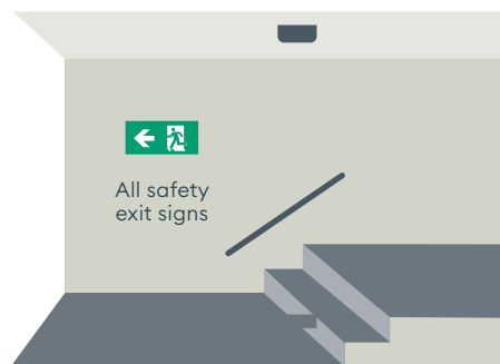
Near stairs so that each tread receives direct light. Also near any change of floor level
